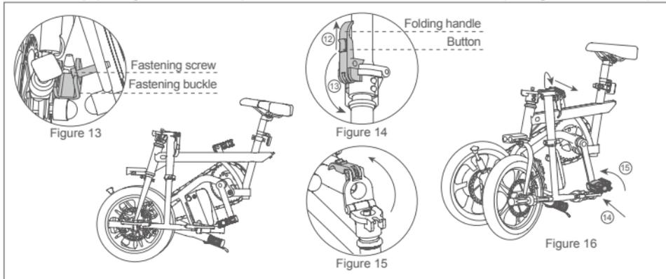
② Put the fastening screw in the fastening buckle (see Figure 13). Push up the button on the handle (see figure 14- ⑫ arrow) and fold down the folding handle (see figure 14- ⑬ arrow). Fold the head as shown in Figure 15. Push the pedal up and inward (see figure 16- ⑭ arrow and ⑮ arrow) to fold the pedals.
