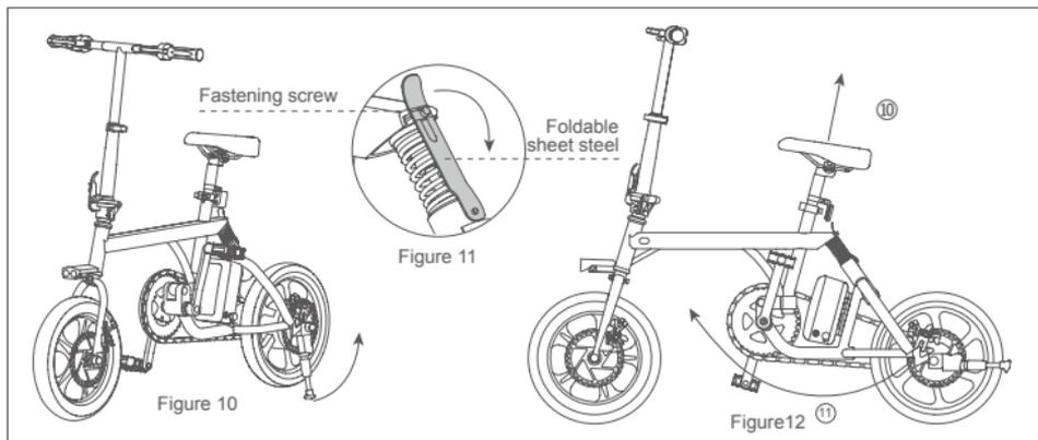
① Adjust the heights of the bike head and saddle to the lowest and fold the kick-stand (see figure 10). Open the folding steel sheet to separate the folding steel sheet and fastening screw (see Figure 11). Pull the saddle up (see figure 12- ⑩ arrow) and rotate forward the rear wheel to fold (see figure 12- ⑪ arrow).
