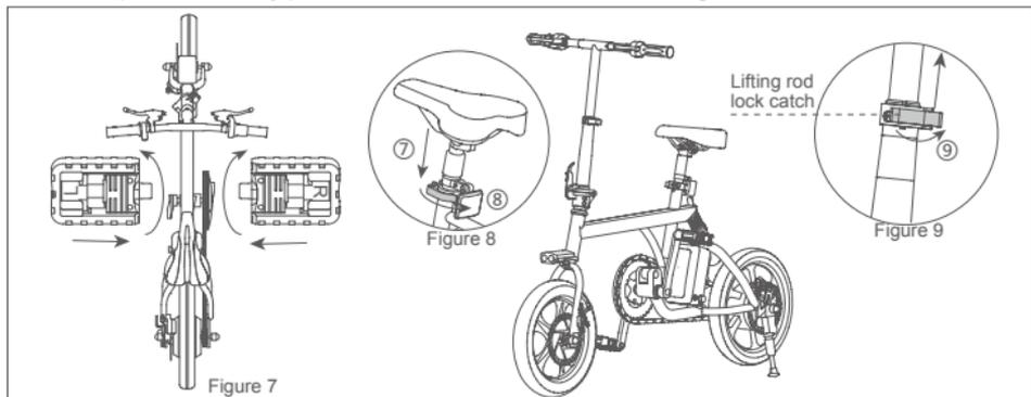
② Install the pedals correctly (L-left, R-right) as showed in Figure 7. Please note the installation of screw tooth is the opposite. Install the left pedal anticlockwise and right pedal clockwise. 35~40N.m is the recommended torque. Adjust the saddle height and install it (see Figure8- ⑦ arrow) and close saddle's lifting rod lock (see Figure8- ⑧ arrow). Open the lifting rod lock and adjust the head height (see Figure9- ⑨ arrow) and close saddle's lifting rod lock.
